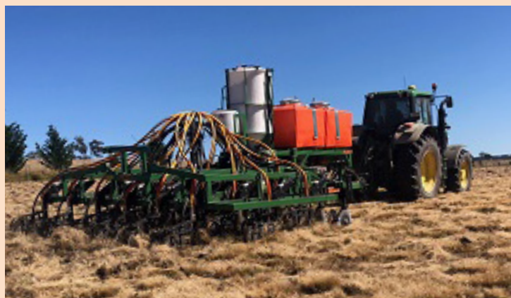
Glen Innes farmer Greg Chappell, NSW, took this photo of his made-to-order DBS and Multistream liquid-ready air seeder, planting Colossus oats at 60kg/ha
